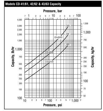
Capacities given are continuous discharge capacities in pounds and kilograms of hot condensate per hour at pressure differential indicated with condensate temperatures approximately 25°F (14°C) below steam temperatures.
